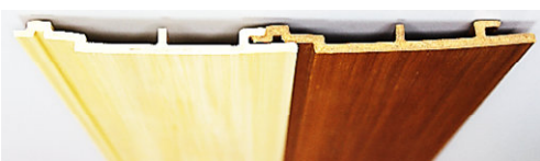
"EAZY-CEIL 12121" 12 thk. x 121 x 3,050 mm (T&G with ~ 7mm width groove)
